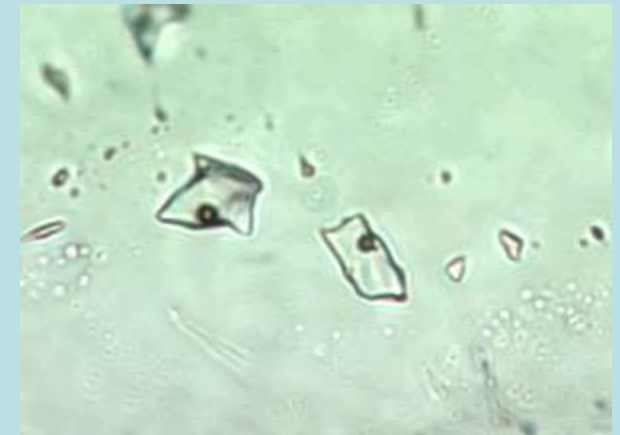
2-phase aqueous inclusions; methane inclusions occur in associated quartz
